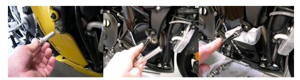
5. Using one drop of blue thread locker mount the right side puck to the offset with 99-HB-SH10125060 Socket Cap 10 X 1.25 X 60 (Holds puck to offset). Torque down to 33 to 35 foot lbs.
