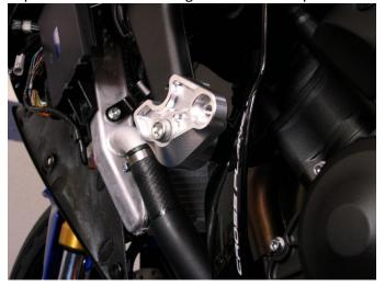
3. Using one drop of blue thread locker mount the left side puck to the offset with 99-HB-SH10125060 Socket Cap 10 X 1.25 X 60 (Holds puck to offset). Torque down to 33 to 35 foot lbs.
