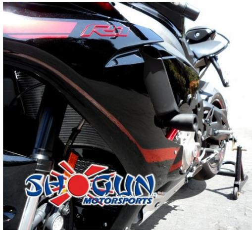
2. Remove the right side bolt. Mount the right side puck with (99-HB-SH12125060) Socket Cap 12 X 1.25 X 60 Main Engine Stud and torque down to the OEM recommended torque specifications.
