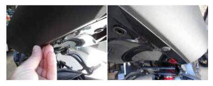
10. Loosely mount the DMP fender kit using the four 8x1.25x30 mm bolts, eight 8mm washers and four 8mm lock nuts. Once the plate is loosely mounted, tighten the plate caddy corner until it's tight. (remaining hardware is for mounting the license plate)
