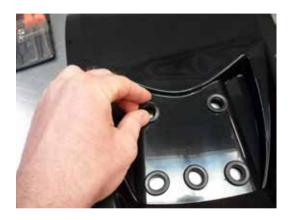
9. Remount the entire tail section and fender following step 6 in reverse. Make sure the fender rivets are put in place and the tail light is plugged in.
