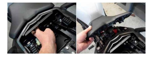
2. Un bolt the four bolts that are holding the OEM fender in place.
