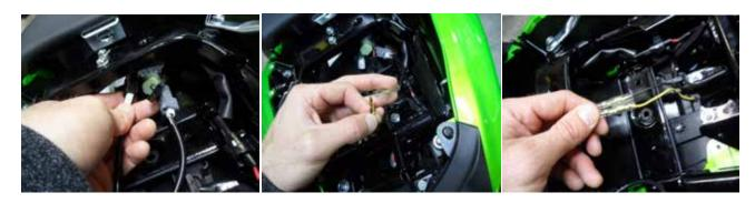
13. Mount your license plate using the two DMP plate lights (900-2042) and hardware. Feed the wires through the center hole of the DMP fender eliminator. We prefer to use the stock plate light connector and wires. Cut the OEM plate light wires to length one at a time. Crimp the butt connectors supplied and pull on each wire to make sure there is a solid connection.
