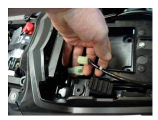
5. Remove the wire covers and un plug the turn signal and plate light connections. Make sure you identify and mark off the left and right turn signals as well as the plate light positive and negative.
