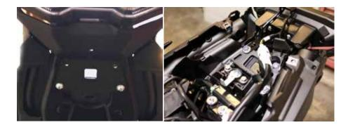
9. Mount the license plate bracket using two 6x25 bolts, two 6x12 washers, two 6x15 washers and two 6mm locknuts. The larger washers and nuts mount inside the tail section.
