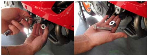
6. Line up the edge of the offset (wile mounted) with the edge of the frame and torque down to OEM torque specs using the stock OEM 12mm Hex Flange bolt. Make sure that the coolant line is secure, routed properly and is not being pinched by the offset or clutch cable in anyway.
