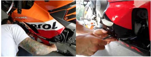
On the left side use one drop of blue thread locker on the (99-HB-SH10125080) Socket Cap 10 X 1.25 X 80 (Holds puck to offset). Torque down to 30 to 32 foot lbs. On the right side use one drop of blue thread locker on the (99-HB-SH10125070) Socket Cap 10 X 1.25 X 70 (Holds puck to offset). Torque down to 30 to 32 foot lbs.
