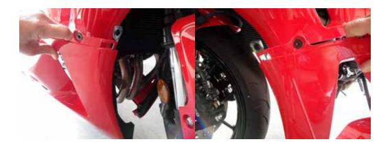
2. Remove left engine stud. There is a spacer that is located between the frame and the engine. Your left side offset will mount in this location.
