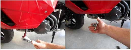
3. Mount the left side offset using the stock OEM 12mm Hex Flange bolt. Make sure that the wire loom is routed properly and not being pinched by the offset in anyway.Line up the edge of the offset (wile mounted) with the edge of the frame and torque down to OEM torque specs.
