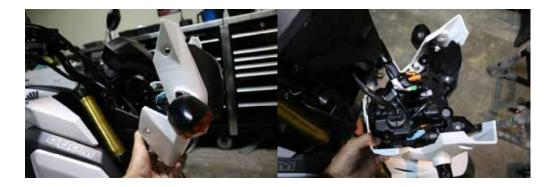
19. Locate and remove the OEM flasher relay.
