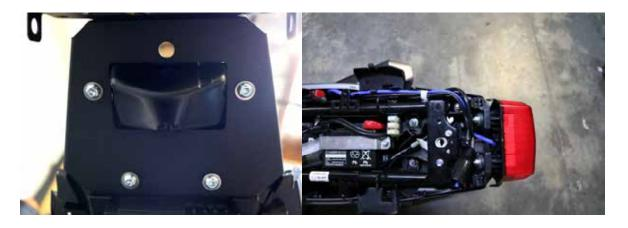
8. Remove the wire cover to expose the turn signal and plate light wires on the OEM fender (screws circled in Red).
