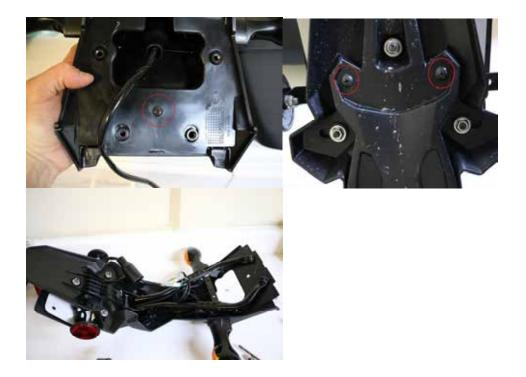
9. Disconnect the turn signal wire bullet connectors (If you are using a DMP plate light, you will need to cut the plate light wires as close to the stock plate light as possible. Splicing is required). Reconnect the turn signal wire harness to the male side on the bike.
