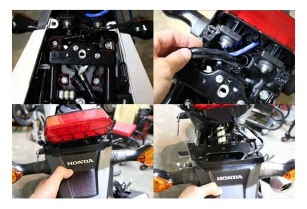
7. Mount the DMP Fender Eliminator Bracket using the four 99-HB-8x20 bolts, eight 8mm Washers and four 8x1.25 Lock Nuts.
