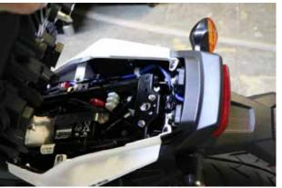
2. Remove the tail section body work screws and bolts (make sure all screws and bolts have been removed).
