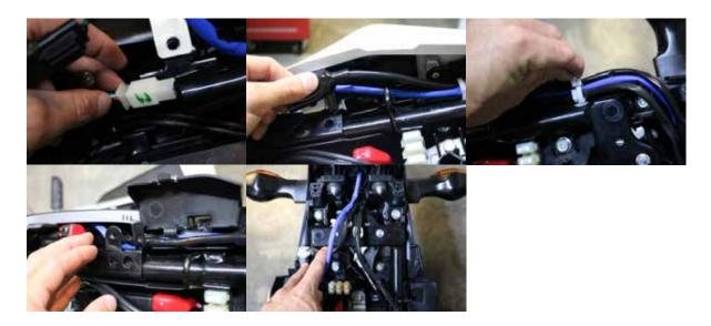
6. Remove the four bolts holding the OEM fender (Circled in Red). Guide the turn signal and plate light wires through the center of the undertail.
