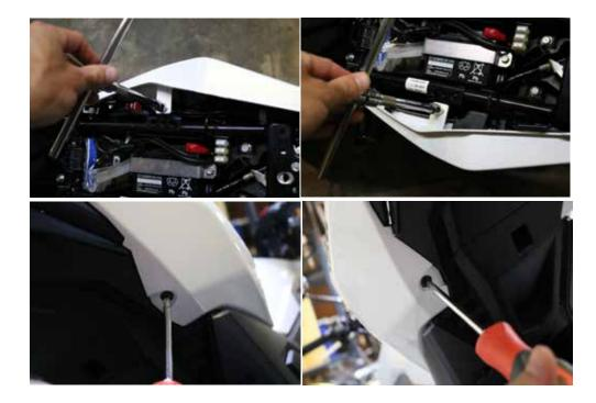
3. Un snap and un plug the tail section body work.
