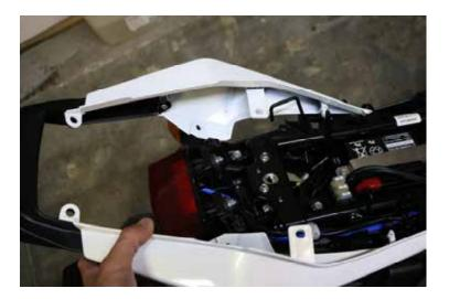
5. Disconnect the turn signal/plate light connector. Remove the wire clamps and free up the turn signal and plate light wires, so they can easily be fed through the center of the undertail for the fender removal.
