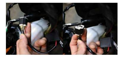
21. The rubber mount for the OEM flasher relay can be used with the DMP Flasher Relay. Make sure the DMP Flasher Relay is securely fastened and mount the head light cover to complete the DMP Flasher Relay install.
