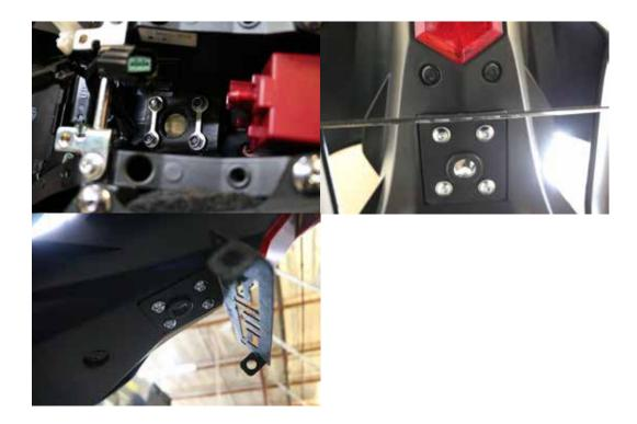
12. Install the desired turn signals and plate lights. We recommend using DMP turn signals and plate lights to complete the install. (OEM turn signals will not work with this application)
