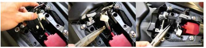
5. Undo the wire clamp holding the turn signal and plate light wires in place.
