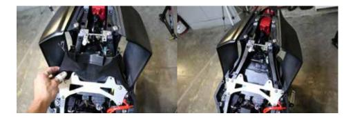
9. Un plug the plate light connections.
