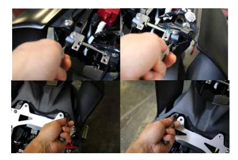
8. Remove the center cowling.
