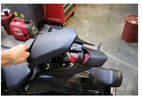
2. Remove the allen head bolts holding the allen keys and turn signal harness in place.
