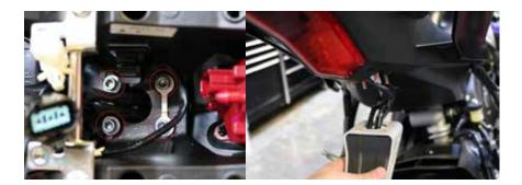
11. Place the supplied rubber grommet (99-FE-GROM562x1.00) around the DMP fender bracket center hole. Mount the DMP fender eliminator bracket using the supplied four 6x1.0x20 bolts and four 6x12 (smaller) washers and four 6x1.0 lock nuts (reuse the OEM fender washers).
