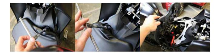
7. Remove the center cowling rivets that are directly behind the rider seat.
