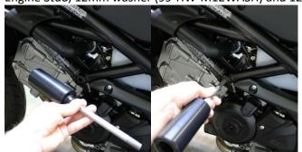
3. Install right side puck along with 12mm washer (99-HW-M12WASH) and 12 X 1.25 lock nut (99-HN-LN12125) and tighten down to OEM torque specs.
