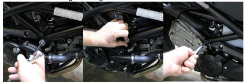
2. Install left side puck along with (99-HR-TH12125398) Threaded SS Rod 12 X 1.25 X 398 Main Engine Stud, 12mm washer (99-HW-M12WASH) and 12 X 1.25 lock nut (99-HN-LN12125).
