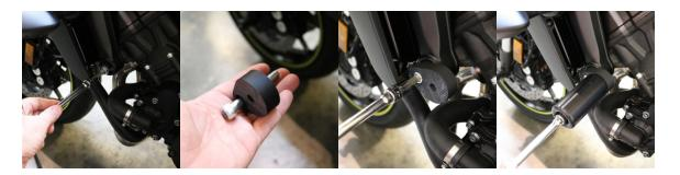
2. Remove right main engine stud. Mount right side offset, orientate offset as shown in the picture below. Using (99-HB-SH10125070) Socket Cap 10 X 1.25 X 70 Main Engine Stud mount offset and torque down to OEM specs. Mount right side frame slider utilizing (99-HB-SH1015045) Socket Cap 10 X 1.5 X 45 (Holds puck to offset) and torque down to 32 FT lbs.
