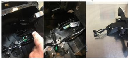
4. Install DMP base plate bracket in conjunction with license plate fender bracket loosely. Use 8 X 20 button heads bolts (4), 8 X 17mm washers (6) 8 X 1.25 lock nuts (4). When mounting the kit use 8mm washers (4) under the button head bolts and the remaining (2) 8mm washers under the locknuts located more towards the front of the bike. Do not use 8mm washers under lock nuts that hold the license plate fender bracket. Tighten up 8mm bolts and lock nuts.
