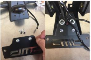
7. Using 8mm hardware 8 X 20 button head bolts, 8mm washers and 8mm locknuts mount the DMP fender kit SLR. Feed wire loom through fender kit reconnect all OEM plugs and test function.
