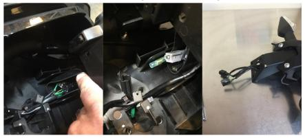
4. Disassemble OEM rear fender to reuse components needed for your DMP fender kit SLR.
