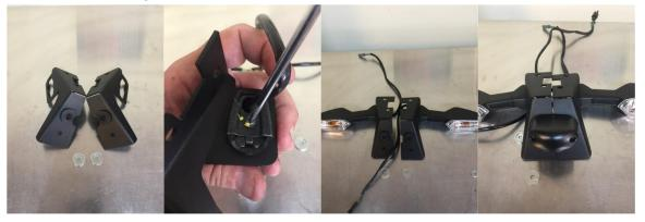
6. Mount DMP license plate holder using 6 X 16 button heads, 6 X 12 washers and 6 X 1 Locknuts.
