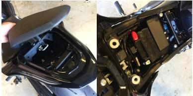
2. Gently remove OEM passenger seat cowling. This step is so you can easily access and disconnect turn signal and plate light connectors required to remove OEM rear fender.
