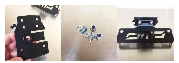
5. Install DMP base plate bracket in conjunction with license plate bracket. Using QTY (4) 6 X 20 button head bolts, black base spacers (428-9180 base spacers are to give clearance between the base plate and tail section), 6 X 15mm washers and 6mm locknuts. Assembly shown below.
