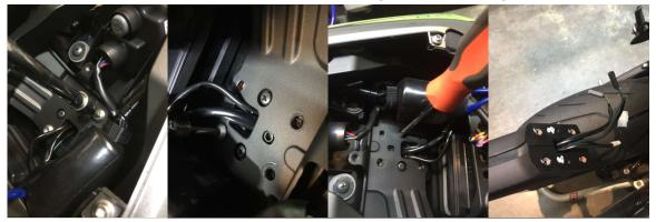
4. Install DMP base plate bracket in conjunction with license plate fender bracket loosely. Use 6 X 30 button heads bolts (4), 6 X 15mm washers (8) 6 X 1 lock nuts (4). When mounting the kit use 6mm washers (4) under the button head bolts and the remaining (4) 6mm washers under the locknuts. Tighten up 6mm bolts and lock nuts. Reinstall actuator bracket.
