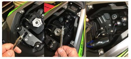
3. Remove OEM fender and disconnect turn signals and plate light.
