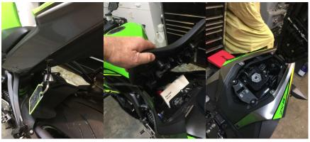
2. Locate and remove actuator bracket to access OEM rear fender.
