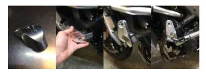
11. With bodywork now removed left and right remove right side OEM engine stud. Make sure you keep track of conical spacers those components will be reused to install right side offset.
