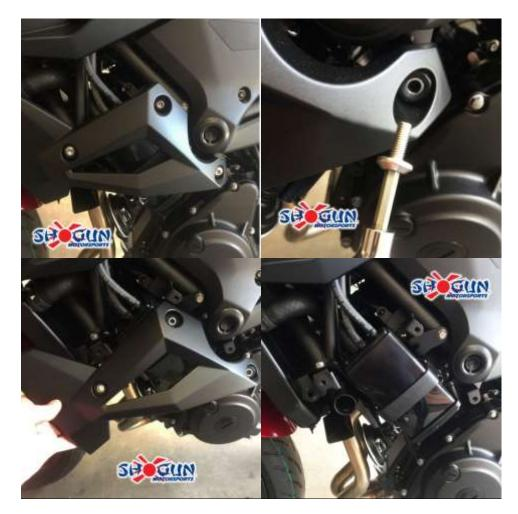
3. Remove left side OEM engine stud. There is a spacer that goes between the frame and the engine.
