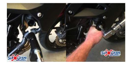
This step is the same for both left and right sliders. Mount left and right sliders using 99-HB-SH10150045 Socket Cap 10 X 1.5 X 45 (Holds puck to offset) one drop of BLUE thread locker and torque down to 32 lbs.
