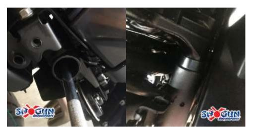
4. Using (SHOGUN Components) the longer of the two spacers (99-SP-428-9175-L left Side Spacer 2.465 Long Black Anodized) the offset 99-OF-428-4150 (both same left and right) and the 99-HB-SH10125140 (Socket Cap 10 X 1.25 X 140) Longer of the two main engine studs assemble the left side components. DON'T FORGET LEFT SIDE OEM STEEL SPACER that goes between the frame and engine. You want to get enough tension on the bolt so you can barely move the offset with one hand.
