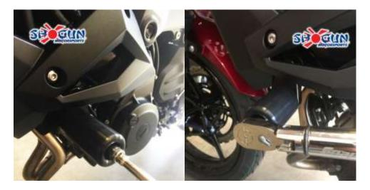
7. Remove right side OEM engine stud.
