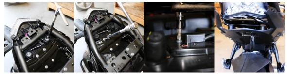
4. Disassemble OEM rear fender to reuse components needed for your DMP fender kit SLR. (Image shown below is a rapid prototype and is for illustration purposes only.)
