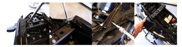
3. Disconnect OEM turn signals and plate light. Loosen fasteners that hold the OEM rear fender and remove.
