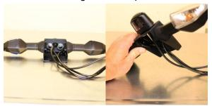
6. Mount DMP SLR Fender Eliminator Kit using 6 X 20 (2) & 6 X 25 (2) button heads, 6 X 15 (8) washers and 6 X 1 (4) Locknuts while pulling OEM wire loom (turn signals and plate light connectors) to the right side of sub-frame, reconnect and test function.
