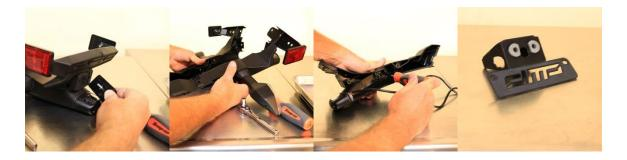
5. Install existing OEM components removed from stock fender to the new DMP fender kit SLR.
