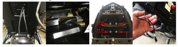
7. Reinstall base fender screws and reinstall side tail section body cowls and seats.
