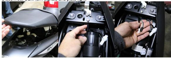
3. Locate and remove OEM rear fender hex flange 6mm bolts. Carefully lower OEM rear fender.
