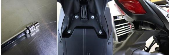
4. Install DMP base plate fender bracket (99-FE-670-5640) utilizing (4) 6 X 12mm (99-BH-6x12) button head bolts, (4) 6x15mm washers (99-Wash6x15) and (4) black washers (428-9170) as shown below.
