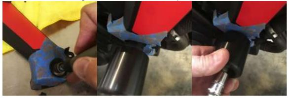
5. With the smaller cowl panel hole cut mate the small cowl with the larger mid cowl. With both panels assembled together scribe a line with a pencil on the inside of the larger mid cowl. With that done disassemble the panels and notch the mid panel along your scribe line.
