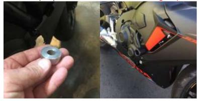
8. Mount left side puck with (99-HB-SH12125090) Socket Cap 12 X 1.25 X 90 Main Engine Stud and torque down.
