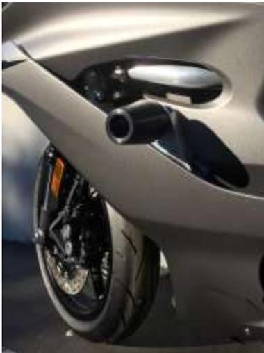
16. Mount right side frame slider using 10 X 1.5 X 45 (99-HB-SH10150045) and torque down to 30ft lbs. **Note: We recommend using one drop of blue thread locker on the end of the threads during install.**
