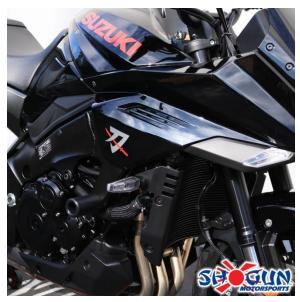
2. Remove left side bolt. Mount left side puck with (99-HB-SH10125080) Socket Cap 10 X 1.25 X 80 Main Engine Stud and torque down to the recommend OEM torque specifications.
